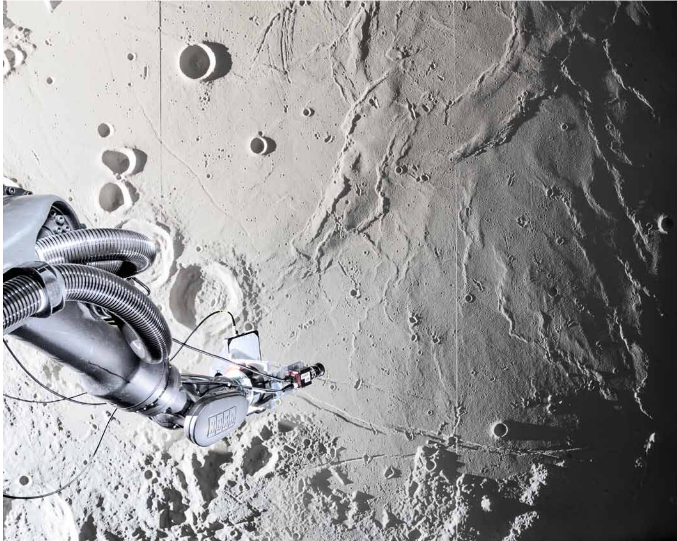
TRON-lab used to simulate optical navigation for landing approaches on moon missions. German Aerospace Centre, Bremen.
