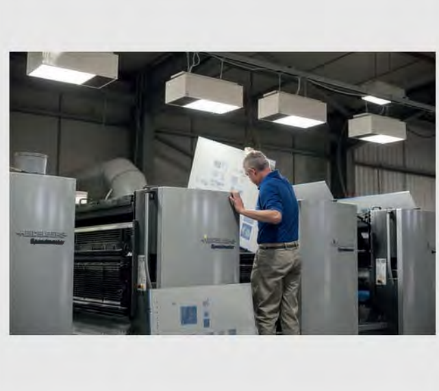
Changing the Plates on the Press
